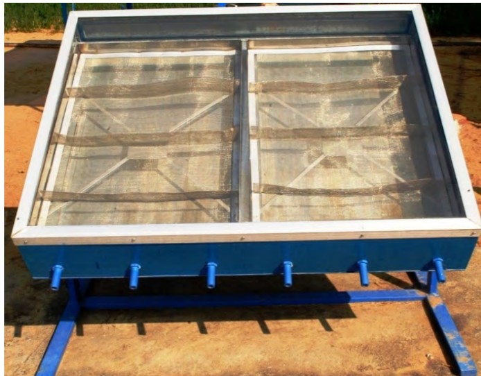
Fig. 2. Inclined solar dryer installed at CAZRI solar yard.
