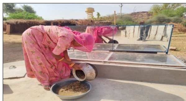
Fig. 5. Animal feed solar cooker.
