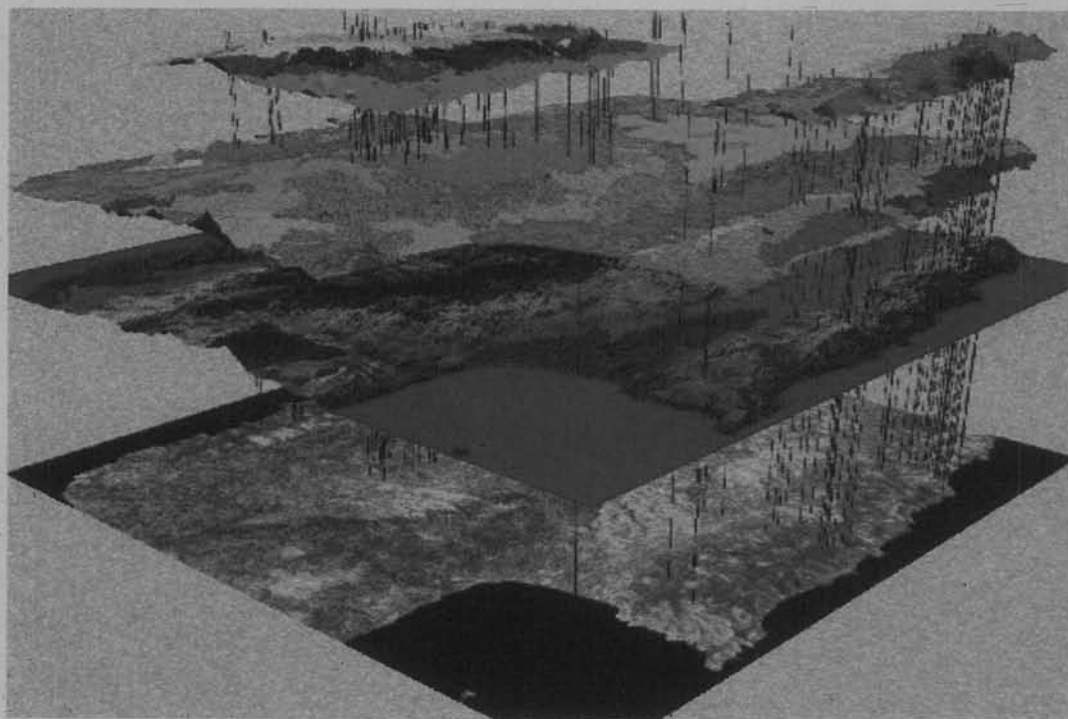
Fig. 6. Integrating vegetation (top) and geology (below) to relate ground measurements (black lines) to features in a DEM or satellite data (bottom).
