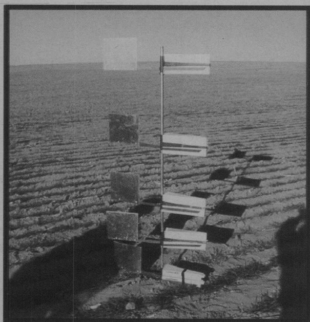
Fig. 3. Station with 6 BSNE samplers. The bottom 2 samplers have smaller openings and share a wind vane.
