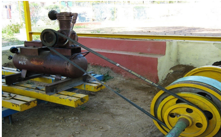
Fig. 7. Testing of air compressor in rotary transmission system.
