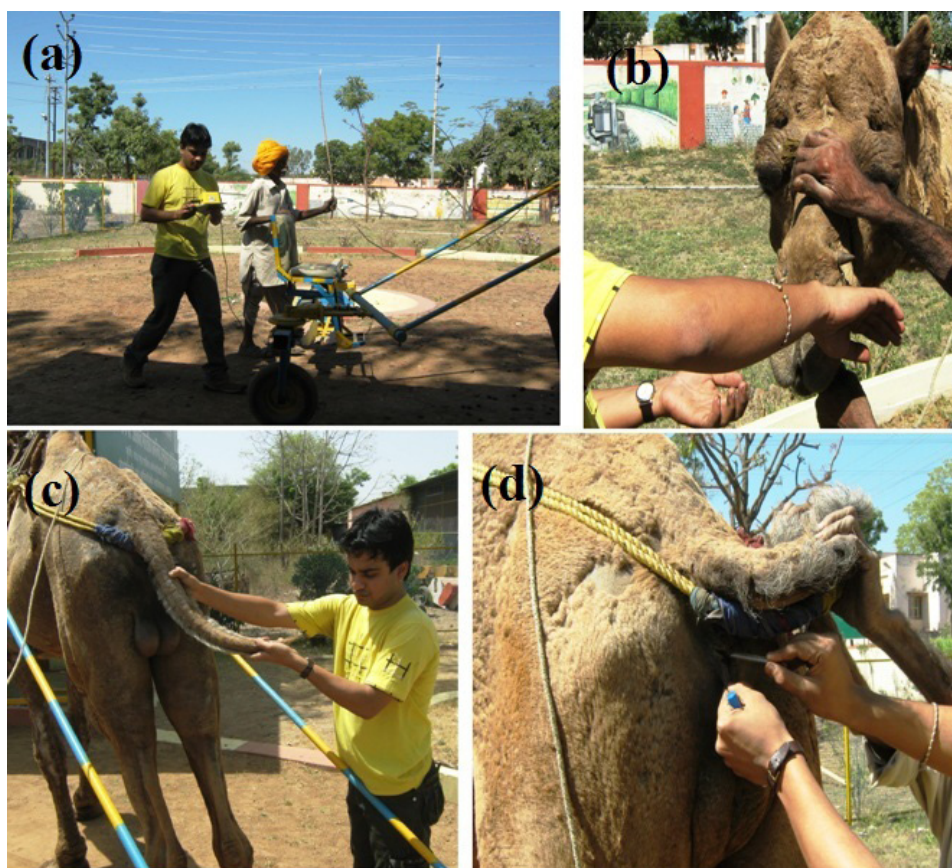
Fig. 9. Measurement of operating and physiological parameters of camel; (a) Measurement of draught, (b) Measurement of respiration rate, (c) Measurement of pulse rate and (d) Measurement of body temperature.
