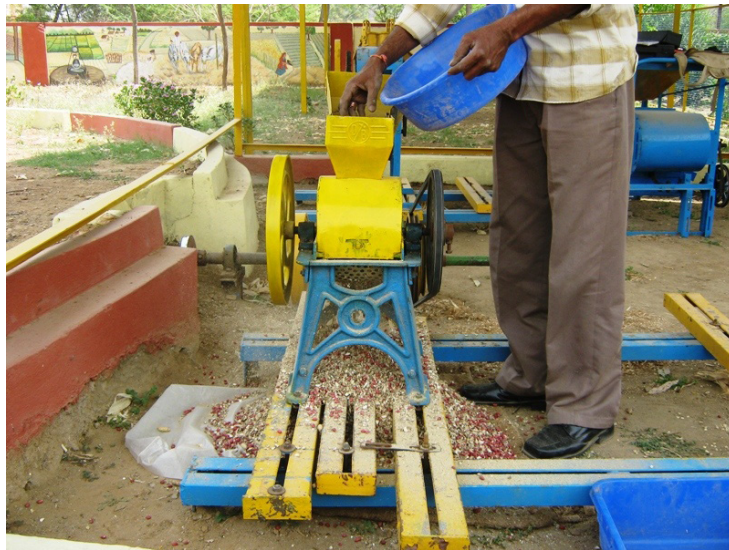
Fig. 6. Testing of groundnut decorticator in rotary transmission system.
