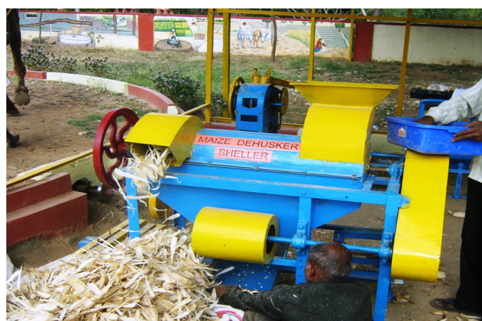
Fig. 5. Testing of maize dehusker sheller in rotary transmission system.
