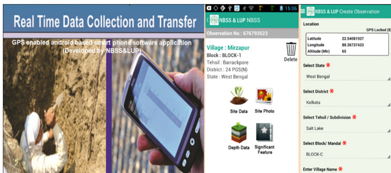
Fig. 7. Android based portable digital assistant for soil survey.
