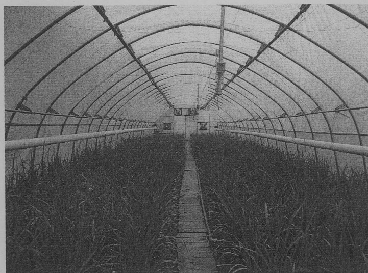
Fig. 2. Photograph of the chamber, showing rice plot, chamber frame with equipments (CO 2 -temperature sensors, fans, blowers and CO 2 pipes).
