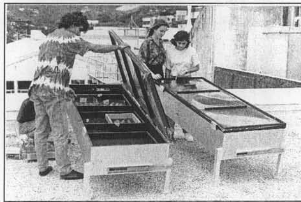
Fig. 5. A direct solar cabinet dryer with side removable drying trays.
