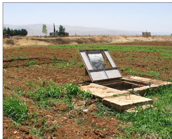
Fig. 1. A view of the weighing lysimeter at Tal Amara Research Station (courtesy: F. Karam, 2005).
