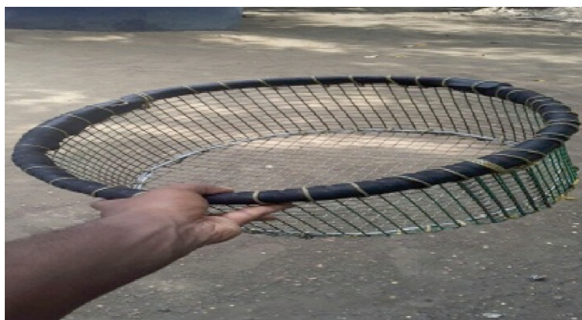
Fig. 2. Type II indigenous device for meat-shell separation
