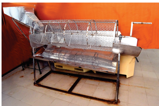
Fig. 5. Fabricated meat-shell separator for clams
