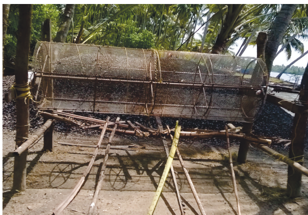
Fig. 3. Type III indigenous device for meat-shell separation
