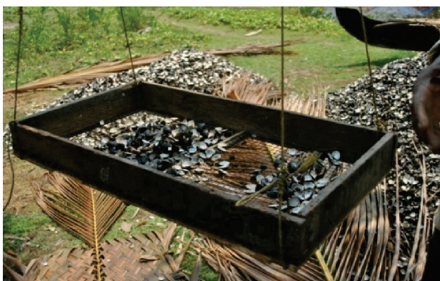
Fig. 1. Type I indigenous device for clam meat-shell separation
