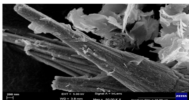
Fig.2. The EDx study of nano-structured FePO 4 ensured its elemental composition and purity (bundle shaped appearance)
