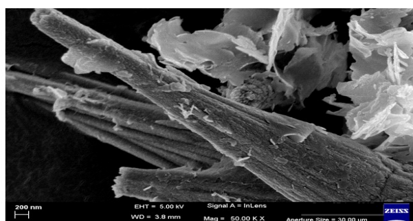
Fig.2. The EDx study of nano-structured \text{FePO}_4 ensured its elemental composition and purity (bundle shaped appearance)
