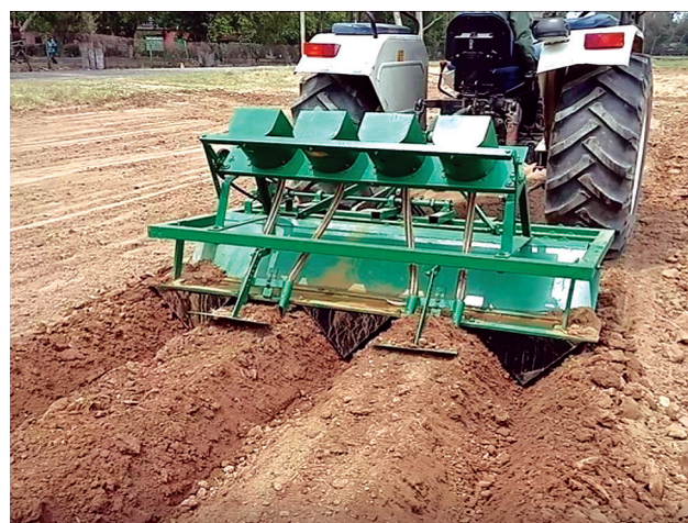
Fig 10 Field testing of developed SR/DR-RB-PP planter
