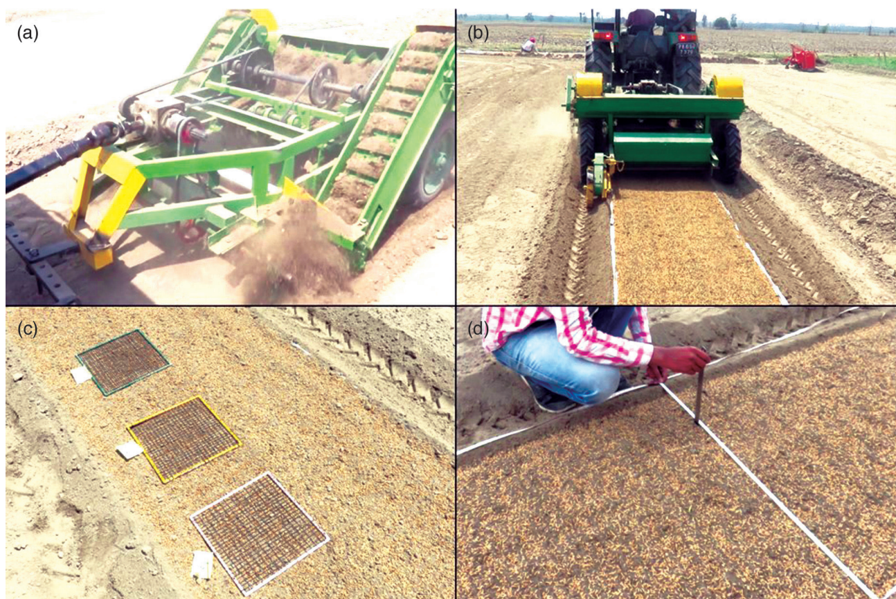
Fig 1 Field evaluation of tractor-operated seeder for mat-type paddy nursery (a) soil placement, (b) seed placement, (c) measurement of seed spread and (d) measurement of soil spread.
