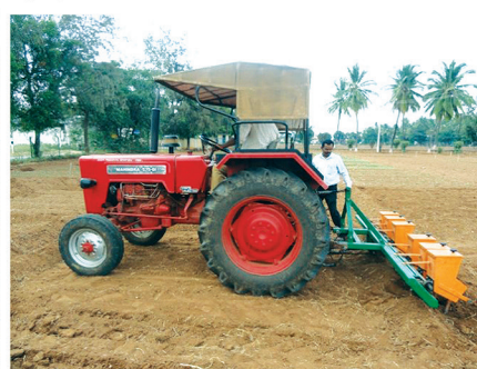
e) CIAE tractor-drawn inclined plate planter (T5)
