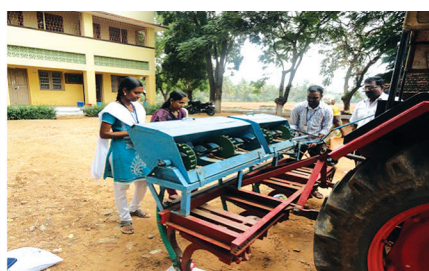
b) TNAU tractor-drawn cultivator-mounted seed-drill (T2)
