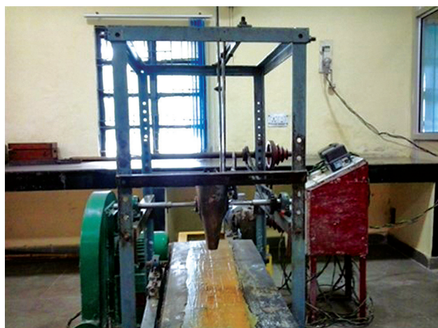
Fig 1 Sticky belt test set-up.
