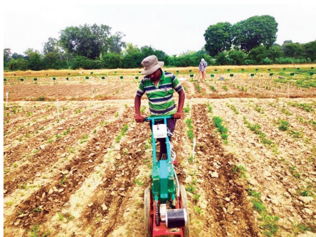
Fig 1 Walk-behind mini electric prime mover for interculture operation.
