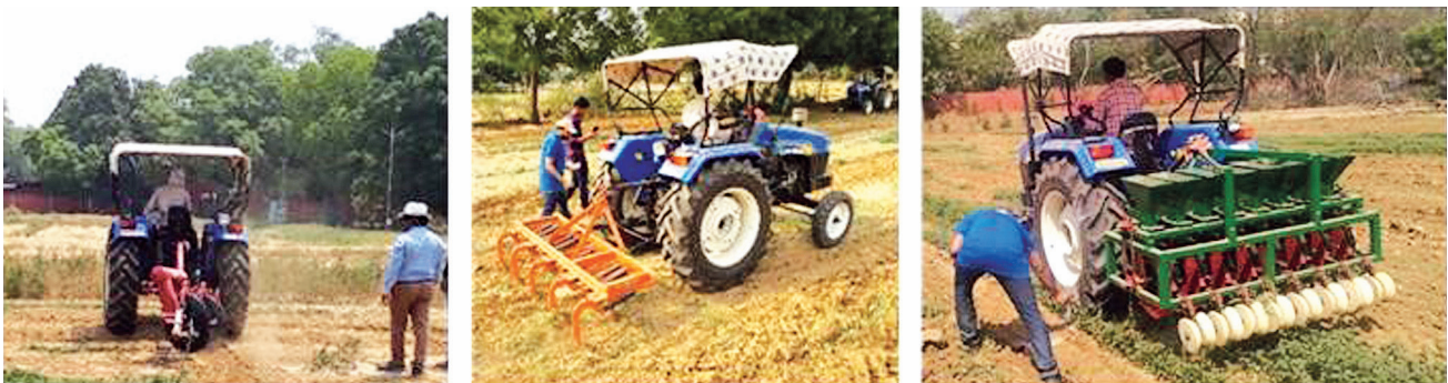
Fig 2 Field experiment for slip measurement with Disc plough, Cultivator and SWI planter.
