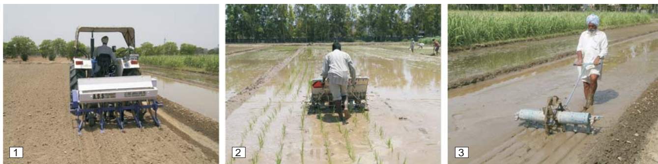
Figs 1–3 1. A view of direct seeded rice drill having inclined plate seed metering mechanism; 2. A view of Japanese paddy transplanter; 3. A view of drum seeder
