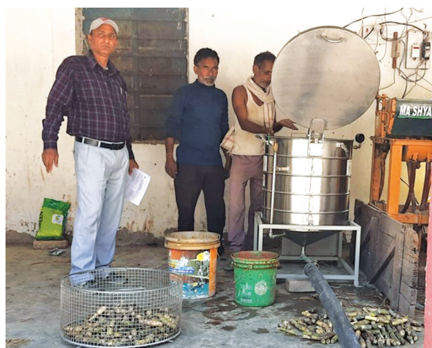
Fig. 1 Treatment of sugarcane setts through sett treatment device.
