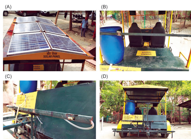
Fig. 3 Different components of solar-operated agricultural vehicle. (A) Solar panel on the roof, (B) Storage compartment for the various tools, (C) Circular sprayers for fertilisers and (D) Sprinklers for irrigation.
