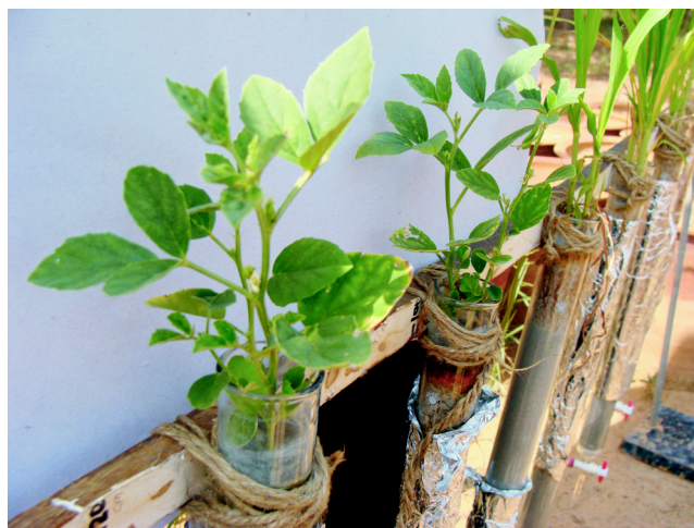
Fig 1 Experimental set up showing pearl millet and clusterbean grown in glass columns
