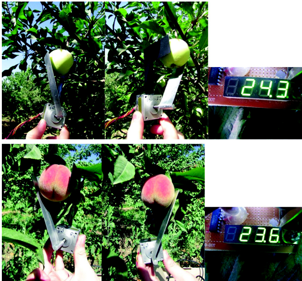
Fig 1 Performance evaluation of the device (left: clockwise rotation, middle: anti-clockwise rotation, right: angular displacement).
