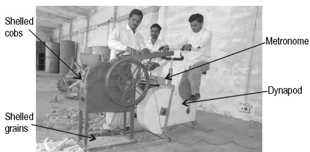
Fig 1 Rotary maize sheller during operation in pedalling mode using dynapod
