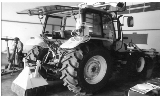
Fig 2 The SOMSENSE and GPS are installed both devices with the computer at the back of this tractor
