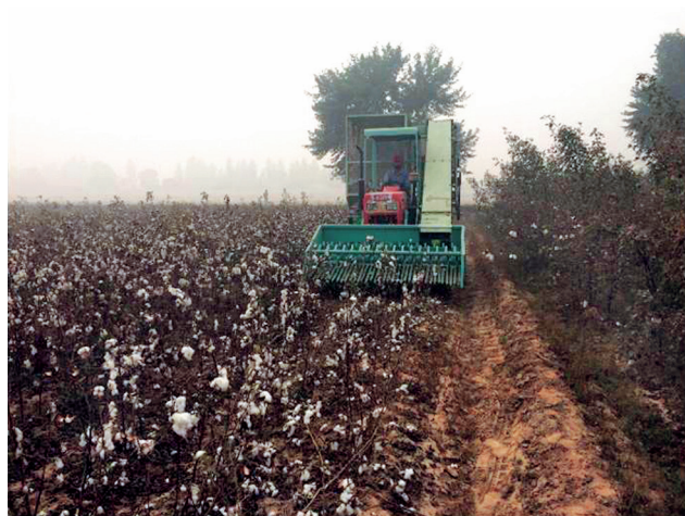
Fig 1 An operational view of tractor operated cotton stripper and harvested field
