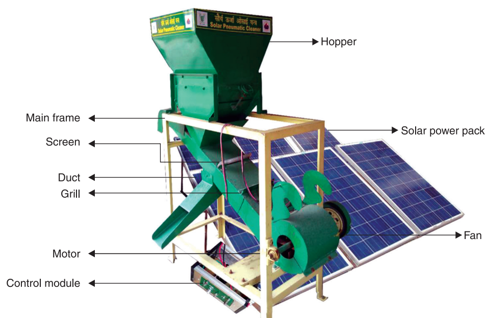
Fig 1 Solar powered pneumatic grain/seed cleaning system.
