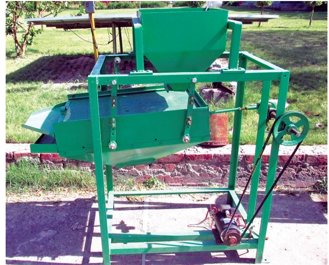
Fig 1 Fabricated unit of solar powered screen cleaner.
