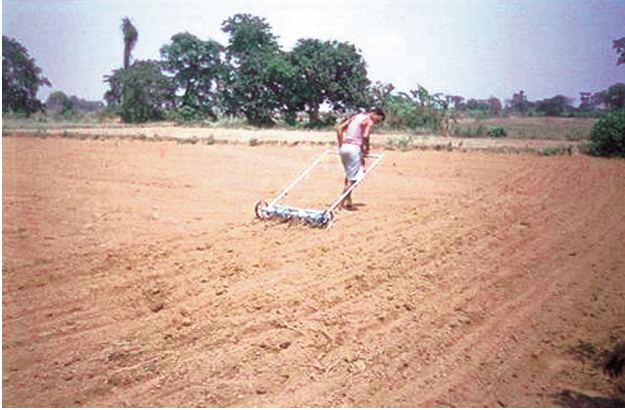
Fig 1 4-rows low cost manual seed drill in sowing operation.
