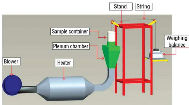
Fig 1 Hot air dryer with continuous sample weighing system.
