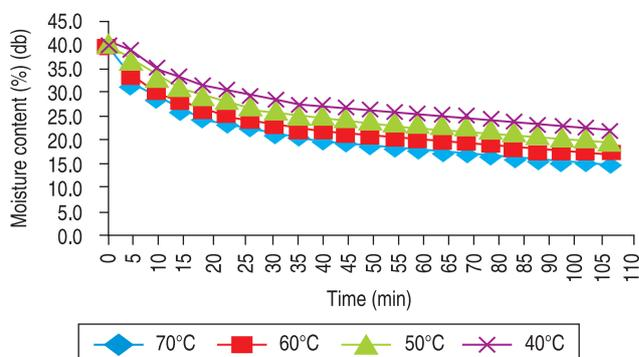
Fig 3 Moisture content vs Drying time for air flow rate of 30 m/min.
