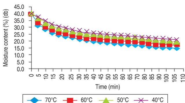
Fig 2 Moisture content vs drying time for air flow rate of 20 m/min.
