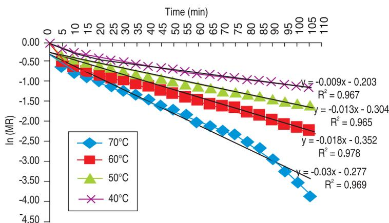
Fig 6 ln (MR) Vs Drying time for flow rate of 40 m/min.
