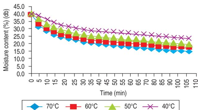
Fig 4 Moisture content vs Drying time for air flow rate of 40 m/min.
