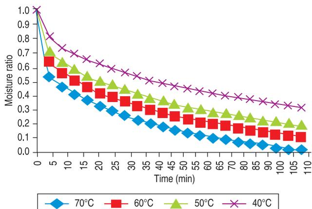
Fig 5 Moisture ratio vs Drying time for air flow rate of 40 m/min.
