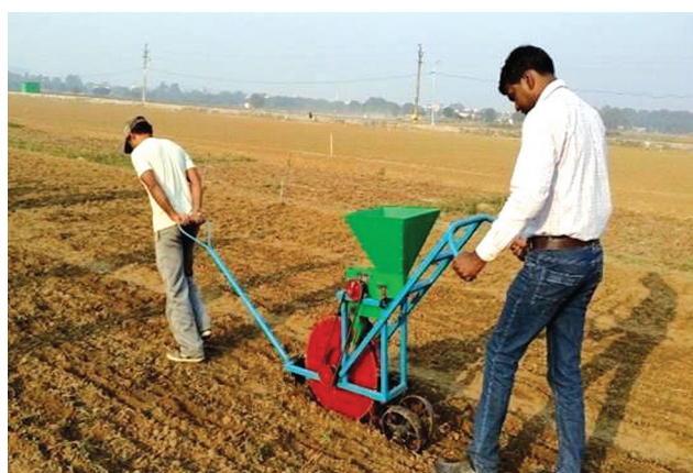
Fig 8 Manual SWI Planter under field trial
