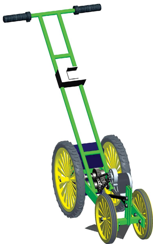
Fig 1 Isometric view of battery-assisted four-wheel weeder.
