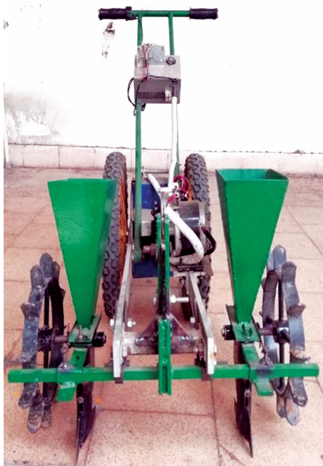
Fig 1 Attached developed seeder on e-powered unit
