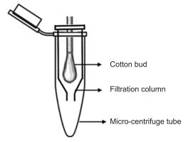
Fig 1. Line drawing of the saliva sample collection device.
