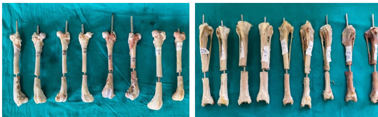
Supplementary Figure 1. Photograph showing bone-pin construct for a fracture gap model in femur and tibia bones.
