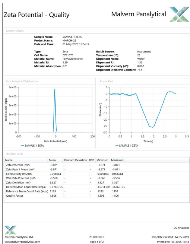
Fig. 3 The zeta size analysis indicated that the synthesised melatonin nanoemulsion is 18.2 \pm 0.1 nm in size with a zeta potential value of -3.87 \pm 0.05 mV
