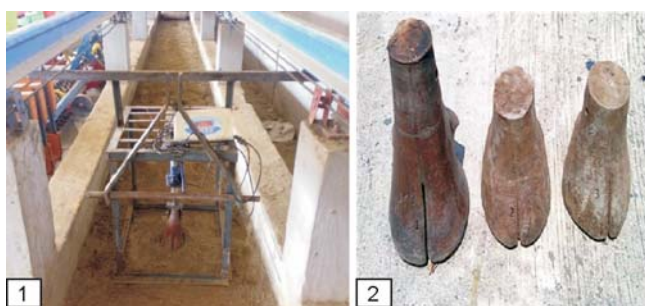
Figs 1–2. 1. Soil bin with test set-up for pressure and sinkage study 2. Artificial wooden legs used in soil bin experiment.
