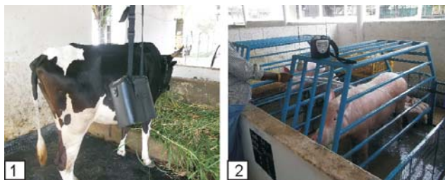
Figs 1–2. 1. Air sampling inside the dairy-shed using multi gas monitor. 2. Air sampling for gaseous pollutants inside the pig shed using multi gas monitor.
