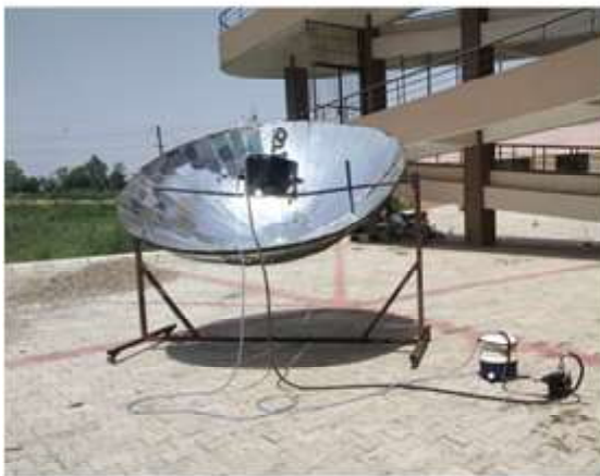
Fig. 2a Set up for solar water heating using paraffin oil
