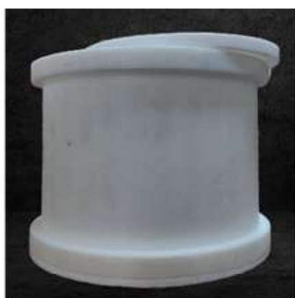
Fig 3e: Developed micro-perforated PTFE mould for paneer pressing
