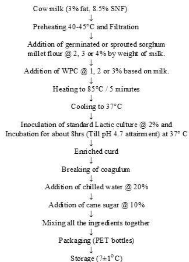
Fig.1 Process flow chart for the manufacture of Sorghum and whey protein concentrate blended lassi
