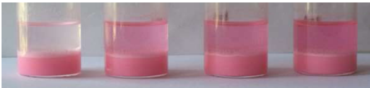
Fig. 2 Qualitative detection of detergent in milk samples using Rhodamine 6G and Toluene solvent
