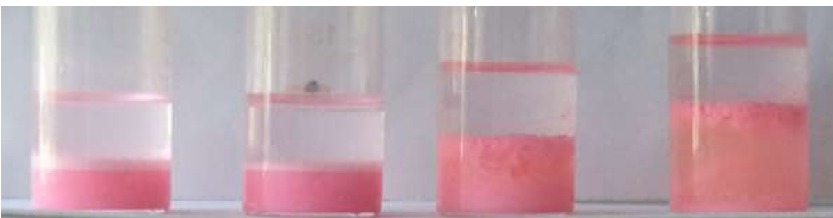
Fig. 3 Quantitative detection of detergent in milk samples using Rhodamine 6G and Toluene
