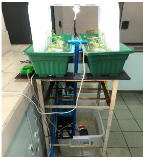
Fig. 5. Aquaponics system with water spinach in the plant boxes with water recycled from the tank at the bottom with freshwater prawns
