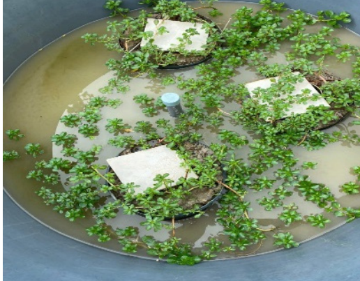
Fig. 3. Ceramic tiles placed over the PVC pipes, with L. adscendens grown on the surface of the barrels
