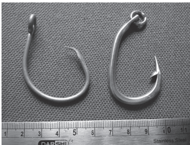
Fig. 1. Hooks used for the study- 14/0 circle hook (left) and 3.5 Japanese tuna hook (right)
