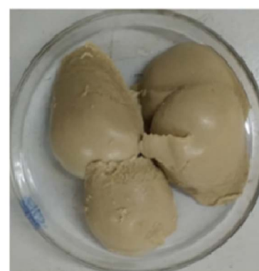
Fig. 3. Fish protein isolate obtained after isoelectric precipitation of solubilised protein
