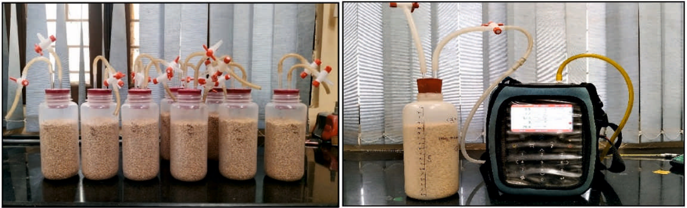
Fig. 3. Experimental setup for CO 2 fumigation to control wheat storage pest R. dominica (Kumar et al. , 2022)
