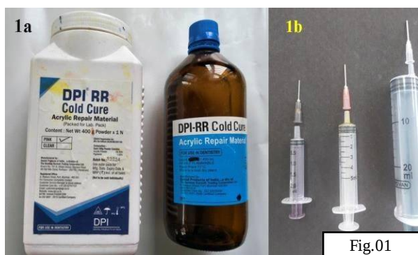
Fig. 1. Photograph showing materials used for corrosion cast method. 1a—DPI RR cold cure acrylic repair material; powder and solvent, 1b—Syringes (5, 10 & 20 ml) with needles (22G, 18G & 16G) respectively. Fig. 2. The kidneys of domestic fowl (Ventral view) along with the blood vessels (2a – kidneys within the renal fossa, 2b—kidneys after excavating from the renal fossa). A—Descending Aorta, B—Cranial renal division, C—Middle renal division, D—Caudal renal division, E—Ischiadic artery, Caudal renal vein (Red colored arrow), External iliac vein (Blue colored arrow), sixth rib (black colored arrow) and seventh rib (Yellow colored arrow).
