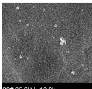
Figure 6: SEM micrograph of silver nanoparticles coated titanium
