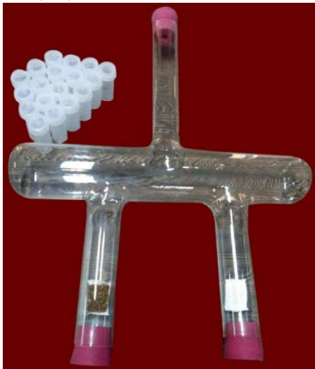
Fig 6. Single cage dual port glass olfactometer for testing food bait preference in house flies
